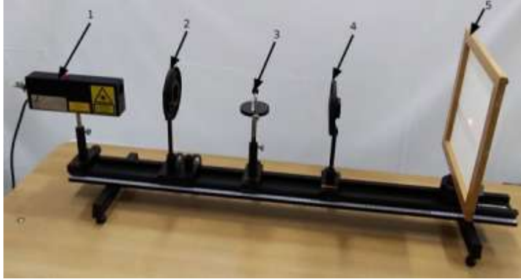
Fig. 12 – The experimental set-up for light interference with the Fresnel biprism. The full color version may be accessed at http://www.rrp.infim.ro/rp/ .
