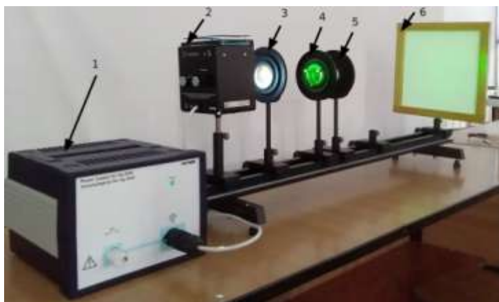
Fig. 2 – Experimental setup for the observation of Newton rings. The full color version may be accessed at http://www.rrp.infim.ro/rrp/ .
