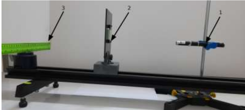
Fig. 18 – Experimental set-up for the diffraction grating. The full color version may be accessed at http://www.rrp.infim.ro/rrp/ .
