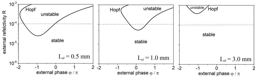
Fig. 6 – Hopf bifurcation in the plane of two parameters (external reflectivity  $R$  - external phase  $\varphi$ ) for different lengths of the active section. The other parameters are the same as in Fig. 5.
