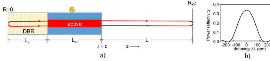
Fig. 1 – a) Scheme of the setup, b) power reflection spectrum of the Bragg reflector of the laser.
