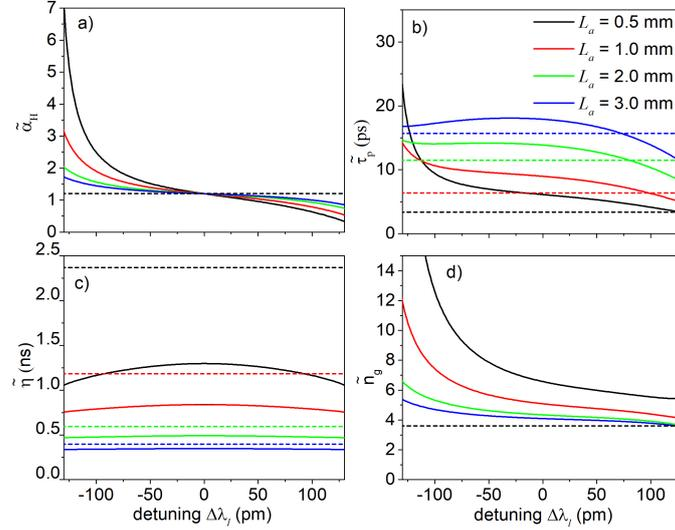
Fig. 2 – The dependence of scaled parameters entering the LK equations on the detuning of the mode of the solitary laser: a) Henry factor  $\tilde{\alpha}_H$ , b) photon life time  $\tilde{\tau}_p$ , c) feedback strength  $\tilde{\eta}$ , and d) group index  $\tilde{n}_g$ . Solid lines: DBR laser, dotted lines: FP laser (see text).
