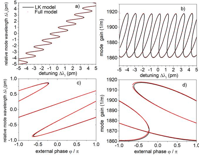
Fig. 4 – Relative stationary wavelength a), c) and stationary gain b), d) versus the relative wavelength of the solitary laser a), b) and the external phase c), d), respectively, for the LK (black line) and full (red dots) models. The length of active section  $L_a = 1.0$  mm and the external reflectivity  $R = 10^{-4}$ . The other parameters are the same as in Fig. 3.
