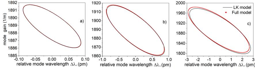
Fig. 3 – Stationary gain *versus* relative stationary wavelength of the LK (black line) and full (red dots) models for different feedback reflectivities. a)  $R = 10^{-6}$ , b)  $R = 10^{-4}$ , c)  $R = 10^{-3}$ . Length of active section  $L_a = 1.0$  mm. Other parameters are as in Table 1.
