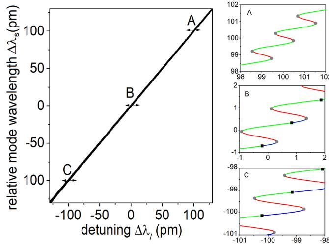
Fig. 7 – Relative stationary wavelength  $\Delta\lambda_s$  versus solitary detuning  $\Delta\lambda_l$  for  $L_a = 1$  mm,  $R = 10^{-4}$ , and  $\varphi = 0$ . Right column: The areas A, B, and C zoomed. The symbols and line colors are the same as in Fig. 5.
