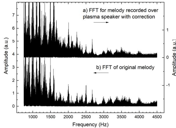
Figure 4 – Comparison of FFT audio spectra recorded over plasma speaker with correction and FFT of original melody.
