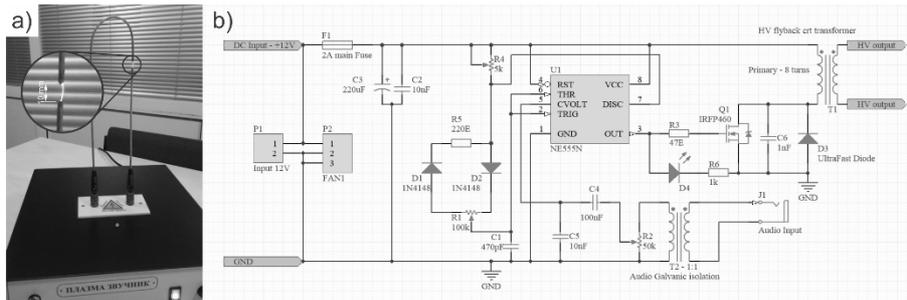
Figure 1 – (a) Laboratory made plasma speaker, and (b) electrical schema used for plasma speaker driver.
