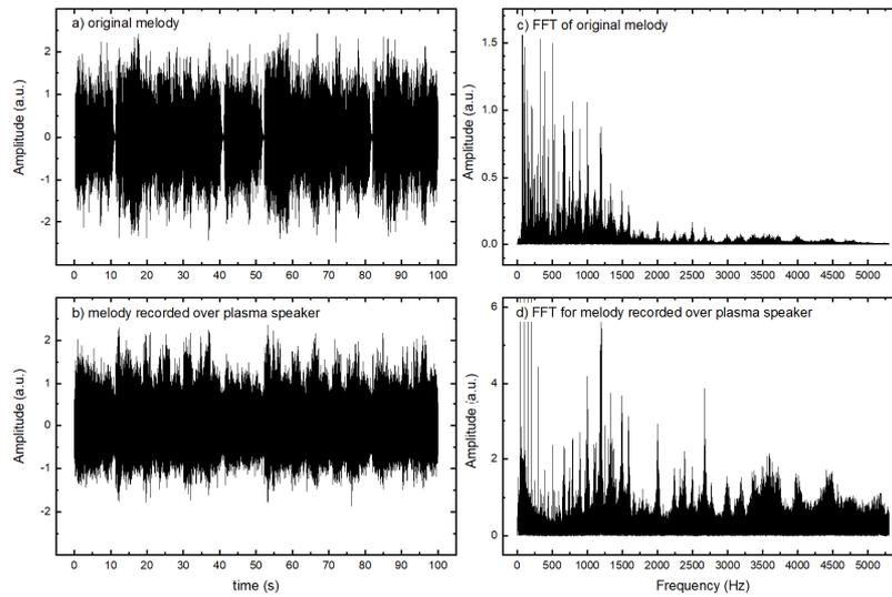
Figure 3 – Comparison of a) audio spectra of original melody and b) audio spectra for same melody recorded via plasma speaker and microphone along with c) FFT of original melody as well as d) FFT for melody recorded over plasma speaker.
