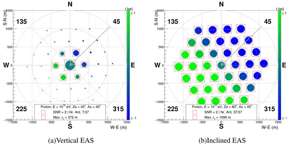
Fig. 2 – Maps of the recorded simulated radio signals for two different shower geometries, highlighting the response of the antennas with SNR above two in open red square markers.
