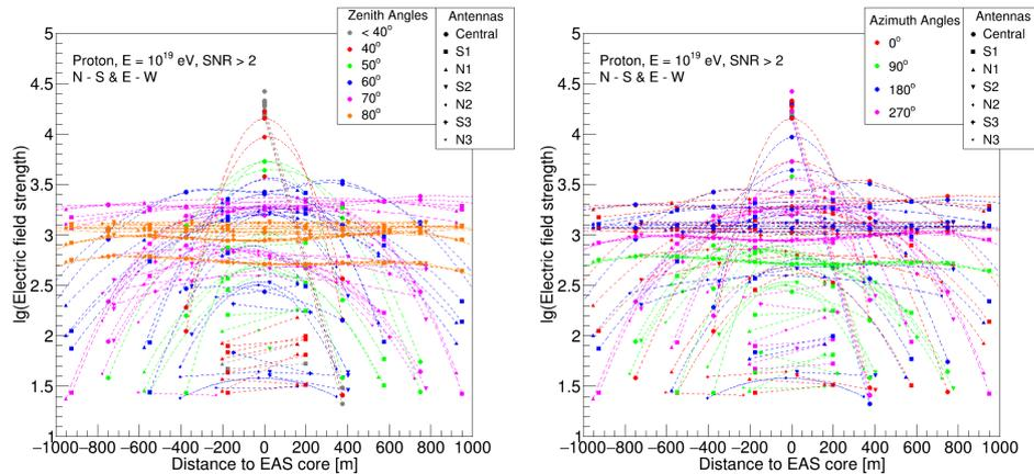
Fig. 4 – The detector response of A37 with seven antenna selections (upwards and downwards to the central horizontal aligned antennas along the East and West directions) for four arrival directions of air showers (North, South, East, West), as function of zenith -left and azimuth -right.
