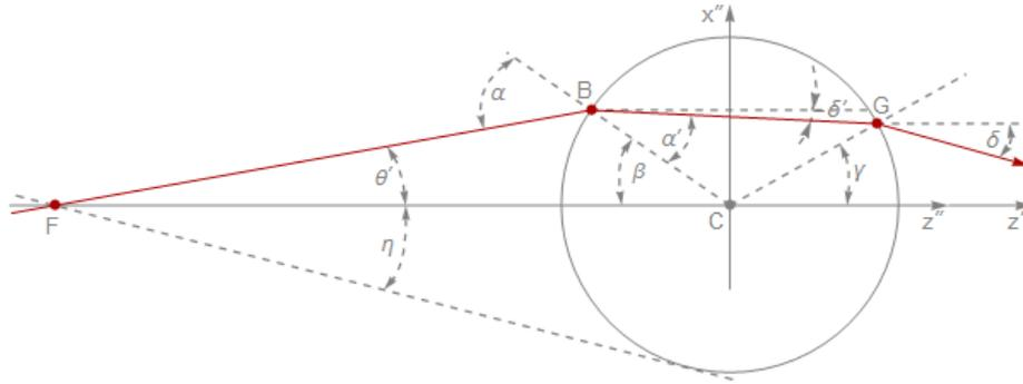
Fig. 5 - Longitudinal section of the system containing the plane  $x''z''$ , without the screen, illustrating the trajectory of the beam through the sphere and the main geometric elements used in the derivation of the formulae.
