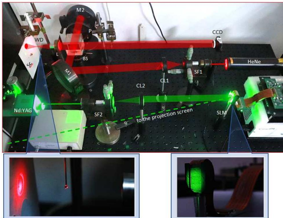
Fig. 2 - Holographic interferometry arrangement. HeNe stands for polarized He-Ne laser (633 nm); Nd:YAG for Nd:YAG second harmonic laser (532 nm); SF for spatial-filter; CL for collimating lens; M for mirror; P for polarizer (light attenuator); BS for beam-splitter cube; WD for water droplet; Sc for white diffusive screen.
