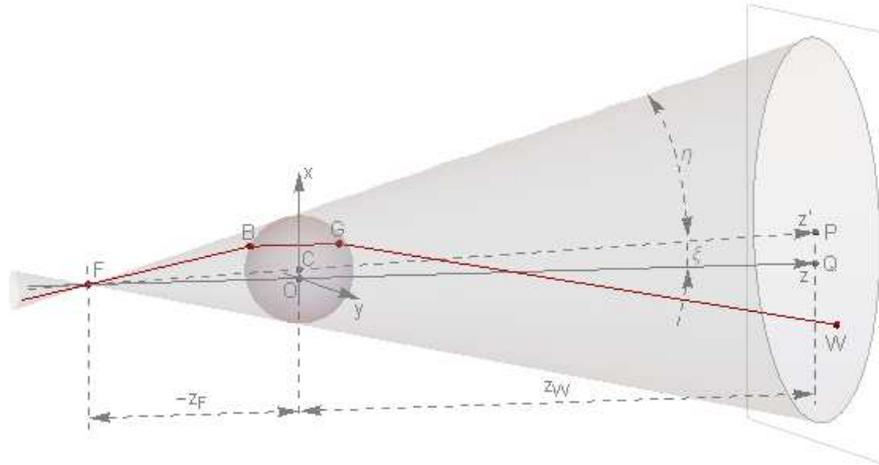
Fig. 3 - Illustration of the general configuration of the divergent beam, the droplet and the screen.  $F$  is the point where the waist of the beam is located,  $C$  the centre of the sphere,  $FBGW$  is an example of ray tracing corresponding to an inclination  $\theta'$  and azimuth  $\varphi$  of the ray.
