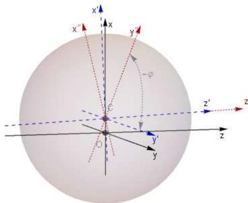
Fig. 4 – Zoom on the droplet, which illustrates the three reference systems used in the analytical derivations.
