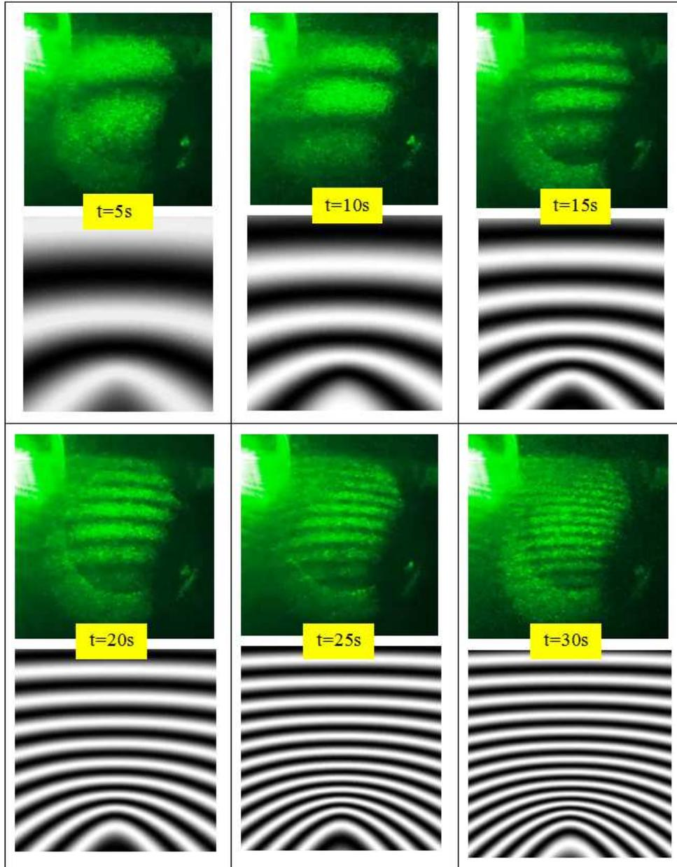
Fig. 6 – Side by side comparison between snapshots of the experimental (green) and the calculated (grey) interferograms taken at 5 seconds intervals during the evaporation.
