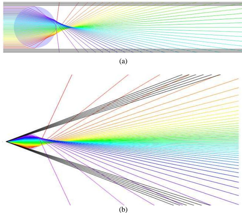
Fig. 1 - A plane-parallel beam is scattered by a water droplet (a). A divergent beam is scattered by a water droplet (b). The light is propagating from left to right. A colour code was used for rays to facilitate the tracking of the rays, namely the rays were coloured from red to violet, starting from the bottom.
