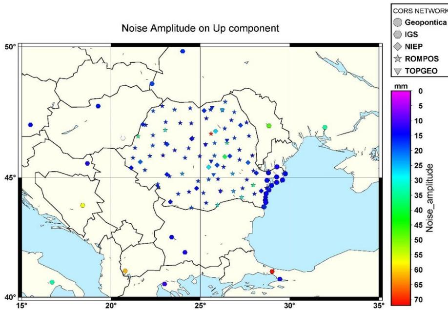
Fig. 4 – Noise Amplitude for the Up component of Romanian GNSS CORS networks.
