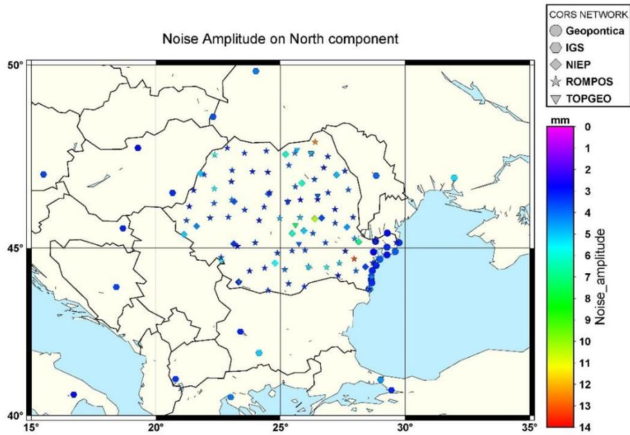
Fig. 3 – Noise Amplitude for the North component of Romanian GNSS CORS networks.
