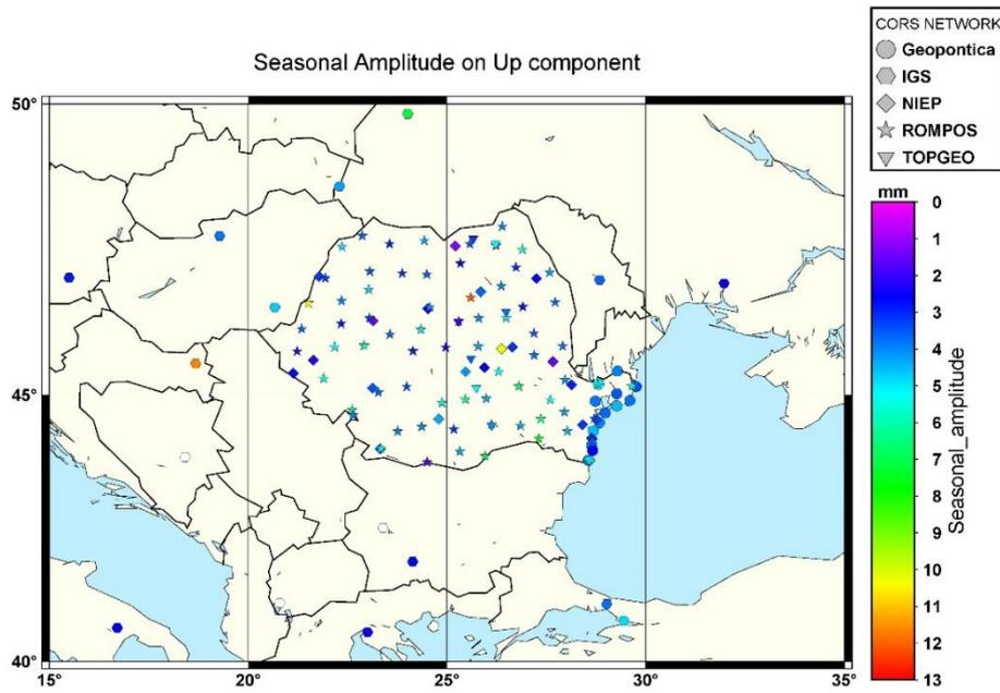
Fig. 7 – Seasonal Amplitude for the Up component of Romanian GNSS CORS networks.
