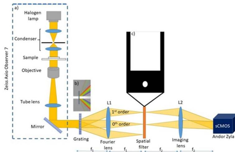
Fig. 1 – Experimental set-up. A transmission grating was placed at the image plane of an inverted microscope, followed by a 4f imaging system. The diffraction orders are collected with a Fourier lens, filtered by a spatial filter, and sent through an imaging lens to the (sCMOS, Andor Zyla, Oxford Instruments) camera.
